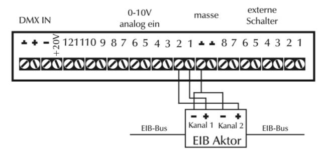
In this example single channels can be dimmed or switched via a standard EIB actor. Alternatively you can connect the actor with the terminals "externe Schalter", to be able, starting the lighting scenes in the dimmer via EIB. For each scene you like to start, there is an actor channel needed. To get a blackout (every channel zero), you have to create an empty scene.
