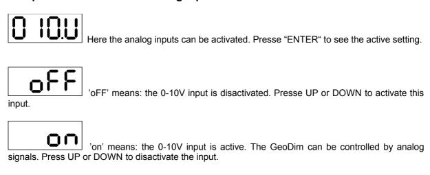
These settings are required, if the analog input will not be used. So signal disturbaces can be separated from the dimmer.
